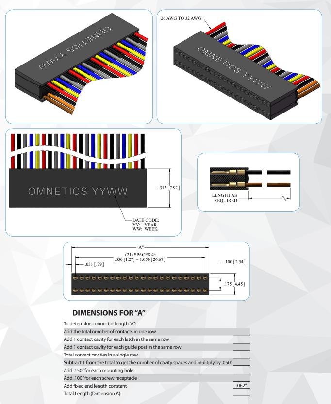
Notes: Maximum length 1.85" (46.99). Maximum number of contact cavities is 64. Number of contacts must be reduced to accommodate hardware and mounting holes. Default locations for guide posts and latches may be changed by customer. Dimensions in [] are in Millimeters unless otherwise noted and are for reference only.
