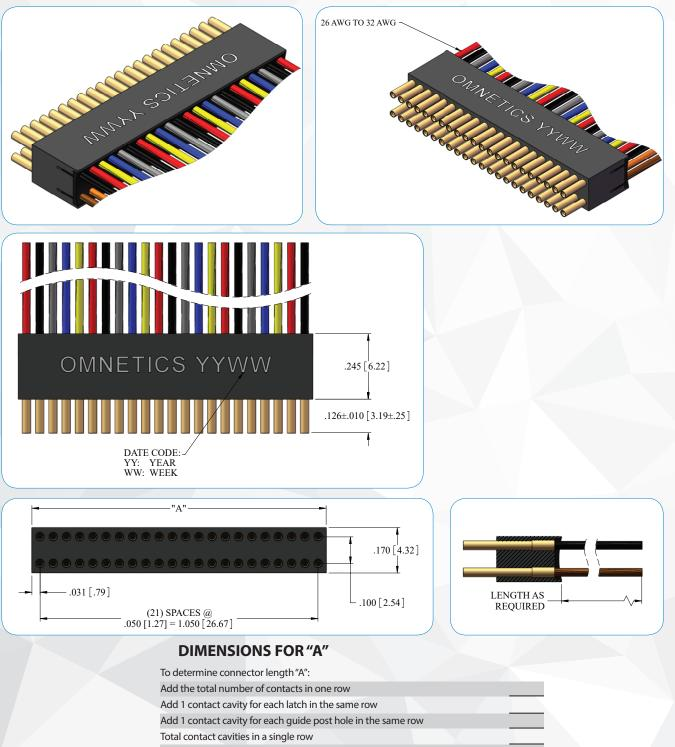
Subtract 1 from the total to get the number of cavity spaces and mulitply by .050" Add .150" for each mounting hole
