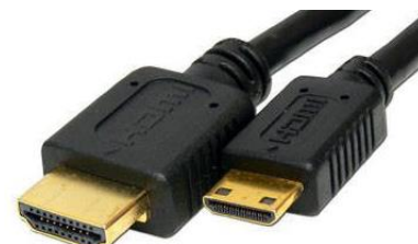
Figure 1. Standard HDMI (Type A), left; Mini HDMI (Type C), right.
