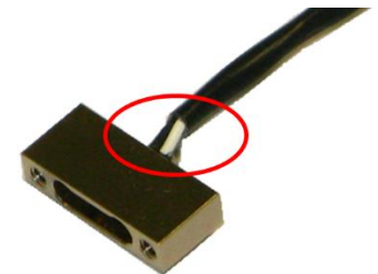
Figure 2. Connector showing wire-pin transition (circled).
